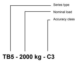
Marking of the knuckle joint: RNS5-2000 kg
