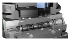
The Axiom's pneumatic valve system consists of a low-power pilot that drives the main highflow spool valve. Pilots may be selected for conventional or bus networking applications. Both stages of the pneumatic valve system have been designed for long life, high tolerance to air line contaminants, and ease of maintenance should components become fouled.
