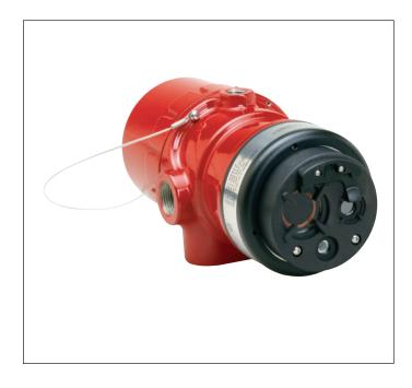
The standard output configuration includes fire, fault and auxiliary relays. An optional 0 to 20 mA output with HART can be provided in addition to the three relays. Auxiliary relay and 4 to 20 mA output are not available with the pulse model. A tricolor LED on the detector faceplate indicates normal condition and notifies personnel of fire alarm or fault conditions.
