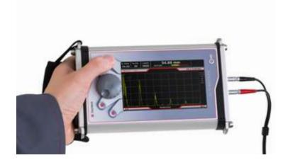
The SONOWALL 70 can be used in two operating modes - wall thickness mode and flaw detector mode. Both software modes can easily be updated vice versa and include:
