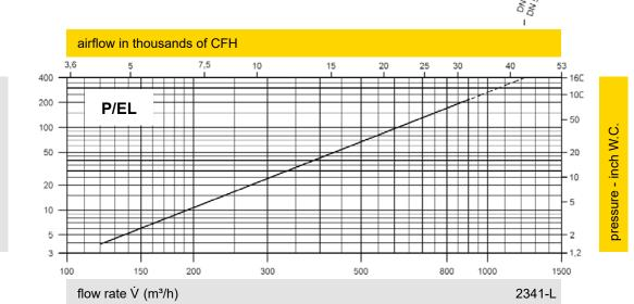
The flow capacity charts have been determined with a calibrated and TÜV certified flow capacity test rig. Volume flow  $\dot{V}$  in (m³/h) and CFH refer to the standard reference conditions of air in ISO 6358 (20°C, 1bar). For conversion to other densities and temperatures, refer to Sec. 1: "Technical Fundamentals."
