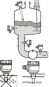
Mounting in pipe forks must be parallel to the direction of flow
