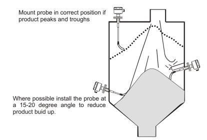
Where possible install the probe away from the inlet to reduce the risk of inflowing material damaging the probe. If the probe is near an inlet, we recommend placing a protective cover 300mm above the probe. The cover should be parallel to the probe and the same length .
