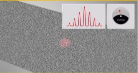
LSV Laser Surface Velocimeters by Polytec use the laser Doppler effect to evaluate the laser light scattered back from the moving object. Two laser beams super-imposed on the surface generate an interference pattern of bright and dark fringes. As the surface moves through the fringe pattern, the intensity of the light scattered back modulates in frequency. This modulation frequency measured by the photo receiver of the sensor system is directly proportional to the surface velocity.
