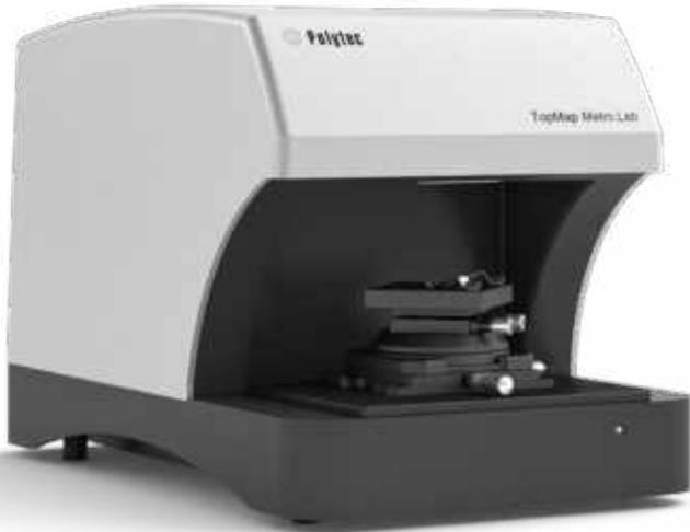
The TopMap Metro.Lab from Polytec is a high-precision white-light interferometer (coherence scanning interferometer) with a large vertical measurement range. The TopMap Metro.Lab is ideally suited for non-contact measurement of flatness, step height and parallelism of large surfaces and structures even on soft or delicate materials.
