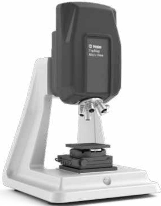
TopMap Micro.View® is an easy to use and compact optical profiler. Combine exceptional performance and affordability with this powerful metrology solution. An extended 100 mm Z measurement range with CST Continuous Scanning Technology allows complex topographies to be measured at nm resolution. This convenient table-top setup features integrated electronics, with the smart focus finder simplifying and speeding up the measurement procedure.
