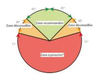
Recommended area: ±45° either side of the vertical axis, bulb down (capillary output up).
