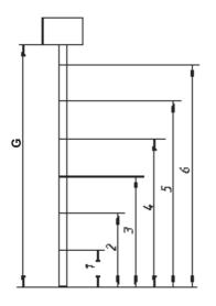
When planning the design of the immersion probes, please consider that when the liquid level rises, the contact of the floating switches is not activated when the floating switches reach the horizontal position, but is activated as depicted in the diagrams of the various floating switches on page 1-1-6 and on the following pages.
