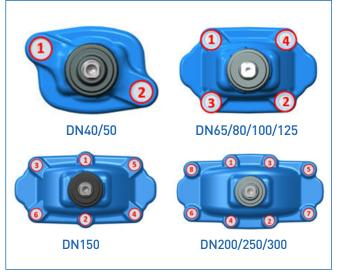
Figure 3: Assembly order for body/bonnet bolts
