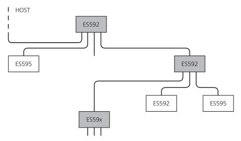
**Fig. 5-5** Example of a Module Network
