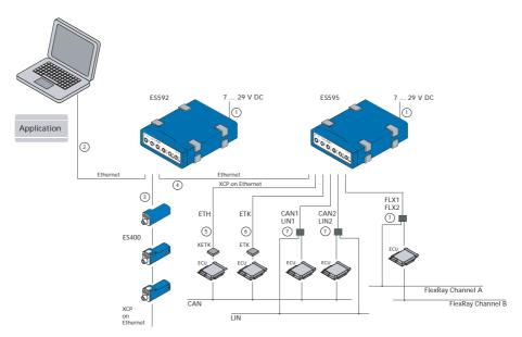
**Fig. 5-4** ES592.1 and ES595.1 with ES400 modules, XETK, ETK and vehicle buses
