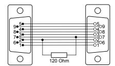
**Fig. 8-18** CBCX131-0 Termination Resistor
