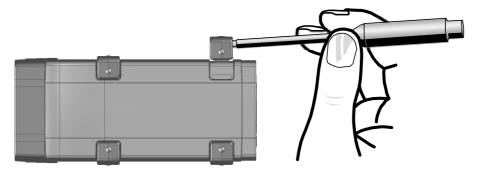
Fig. 5-1 Levering Off the Plastic Foot
