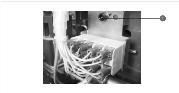
Fig. 14. Aux. switch general view
