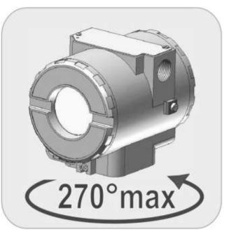
Figure 4.1 – Transducer Rotation Stopper
