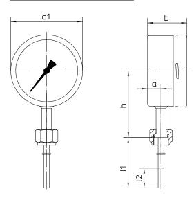
The sensitive portion I2 shall reach the media temperature completely. The insertion length I1 should have adequate size.
