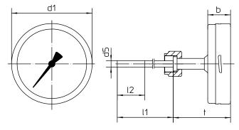
The sensitive portion I2 shall reach the media temperature completely. The insertion length I1 should have adequate size.
