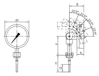
The sensitive portion I2 shall reach the media temperature completely. The insertion length I1 should have adequate size.
