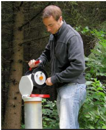
Water level measurement
