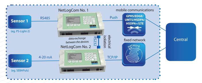
The input channels (W, W1) can be monitored continuously via differential channels in the **NetLogCom**. If the channels drift apart for instance or in the event of an error message (faulty sensor) an instantaneous alarm signal is sent according to the
