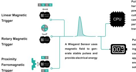
Pulse energy can be harvested to generate power for electronic circuits. Wiegand sensors can additionally serve as part of a wireless power transmission system
