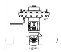
Remove the plastic stopper from the tapped hole in the under side of the bonnet. Install a 1/4" or 3/8" tube fitting (not provided). The tubing must be installed from the source of instrument gas. The plug at the top of the bonnet is a breather plug
