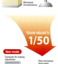
RS232C or RS485 By integrating the microwave-transmission circuit with the signal processor onto three boards, the meter became compact with improved maintainability.
